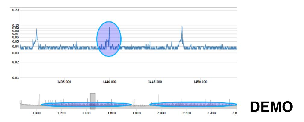
Event-delay pattern caused by mouse movement (on a different tab): 0.1ms delay, 125Hz frequency
